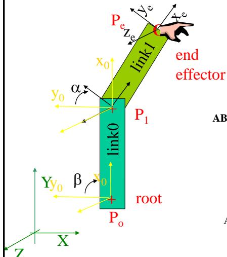
$$\text{ABS\_ABS} \mathbf{P} = \begin{bmatrix} l_1 \cos(\alpha + \beta) + l_0 \cos \beta + T_x \\ -l_1 \sin(\alpha + \beta) - l_0 \sin \beta + T_y \\ 0 \\ 1 \end{bmatrix}$$
