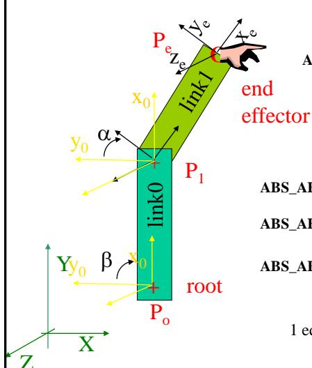
$$\text{ABS\_ABS} \mathbf{P} = \begin{bmatrix} l_1 \cos(\alpha + \beta) + l_0 \cos \beta + T_x \\ -l_1 \sin(\alpha + \beta) - l_0 \sin \beta + T_y \\ 0 \\ 1 \end{bmatrix}$$
