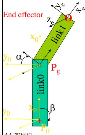
$$\begin{bmatrix} {}^{ABS}_{e}P \\ {}^{ABS}_{g}P \end{bmatrix} = \begin{bmatrix} l_1 \cos(\alpha + \beta) + l_0 \cos \beta \\ -l_1 \sin(\alpha + \beta) - l_0 \sin \beta \\ l_0 \cos \beta \\ -l_0 \sin \beta \end{bmatrix}$$
