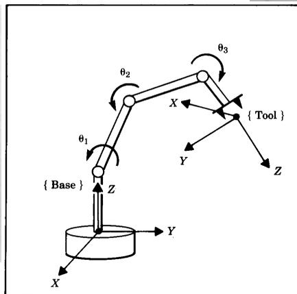
Kinematic chain. Hierarchical structure.
