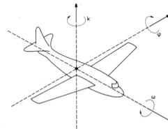
$$\begin{aligned}x_2 &= x' \cos \phi - (-y' \sin \omega + z' \cos \omega) \sin \phi \\y_2 &= y' \cos \omega + z' \sin \omega \\z_2 &= +x' \sin \phi + (-y' \sin \omega + z' \cos \omega) \cos \phi\end{aligned}$$
