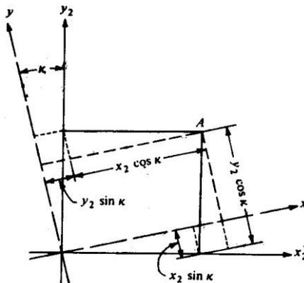
$$\begin{aligned}x_3 &= x_2 \cos k + y_2 \sin k \\y_3 &= -x_2 \sin k + y_2 \cos k \\z_3 &= z_2\end{aligned}$$
