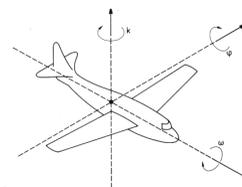
$$\begin{aligned}x_3 &= [x' \cos \phi - (-y' \sin \omega + z' \cos \omega) \sin \phi] \cos k + [y' \cos \omega + z' \sin \omega] \sin k \\y_3 &= -[x' \cos \phi - (-y' \sin \omega + z' \cos \omega) \sin \phi] \sin k + [y' \cos \omega + z' \sin \omega] \cos k \\z_3 &= +x' \sin \phi + (-y' \sin \omega + z' \cos \omega) \cos \phi\end{aligned}$$
