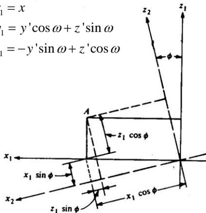
$$\begin{aligned}x_2 &= x_1 \cos \phi - z_1 \sin \phi \\y_2 &= y_1 \\z_2 &= +x_1 \sin \phi + z_1 \cos \phi\end{aligned}$$
