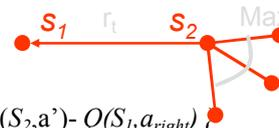
$$\begin{aligned} Q(S_1, a_{right}) &\leftarrow Q(S_1, a_{right}) + \alpha [ r(A, a_{right}, S_2) + \gamma \max_{a'} Q(S_2, a') - Q(S_1, a_{right}) ] \\ &\leftarrow 72 + \alpha [ 0 + 0.9 \max \{ 63, 80, 100 \} - Q(S_1, a_{right}) ] \\ &\leftarrow 72 + \alpha (90 - 72) = 72 + 1.8 = 73.8 \end{aligned}$$
