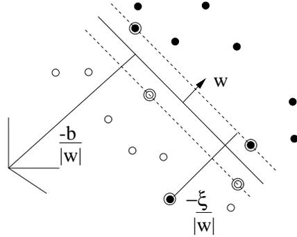
Figure 6. Linear separating hyperplanes for the non-separable case.
