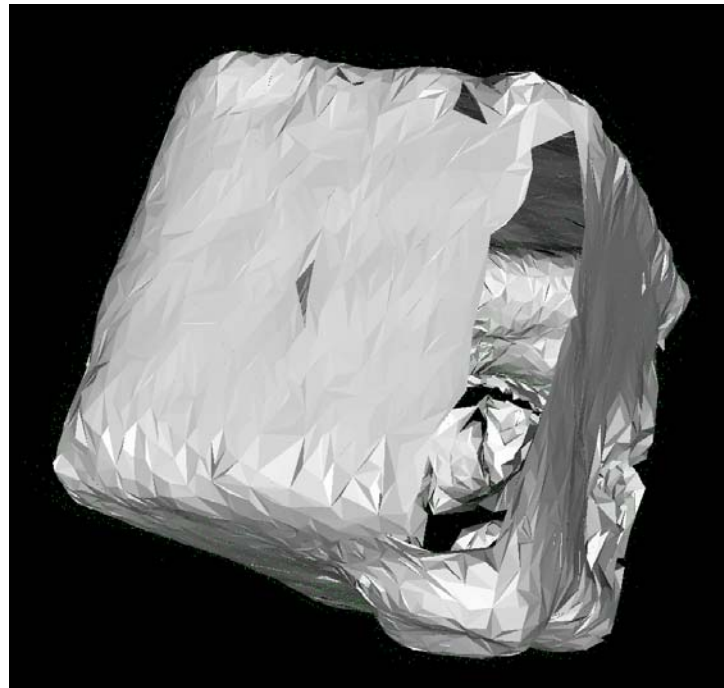
Figure 24 - The edge that leaned against the floor for both object orientations cannot be reconstructed.
