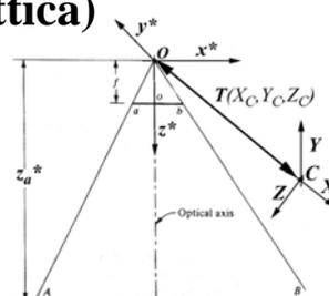
$$x_a - x_o = x_A^* f / z_A^* = f \frac{r_{11}(X_A - X_C) + r_{12}(Y_A - Y_C) + r_{13}(Z_A - Z_C)}{r_{31}(X_A - X_C) + r_{32}(Y_A - Y_C) + r_{33}(Z_A - Z_C)}$$
