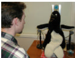
Penguin robot that recognizes and produces gestures (MERL)
