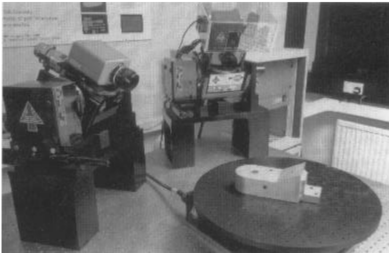
Figure 1.1 A prototype of 3-D inspection cell. The cell includes two types of depth sensors, a laser scanner, and a Moiré fringe system (see Chapter 2), which locate the object in space and perform measurements. Notice the turntable for optimal, automatic object positioning.
