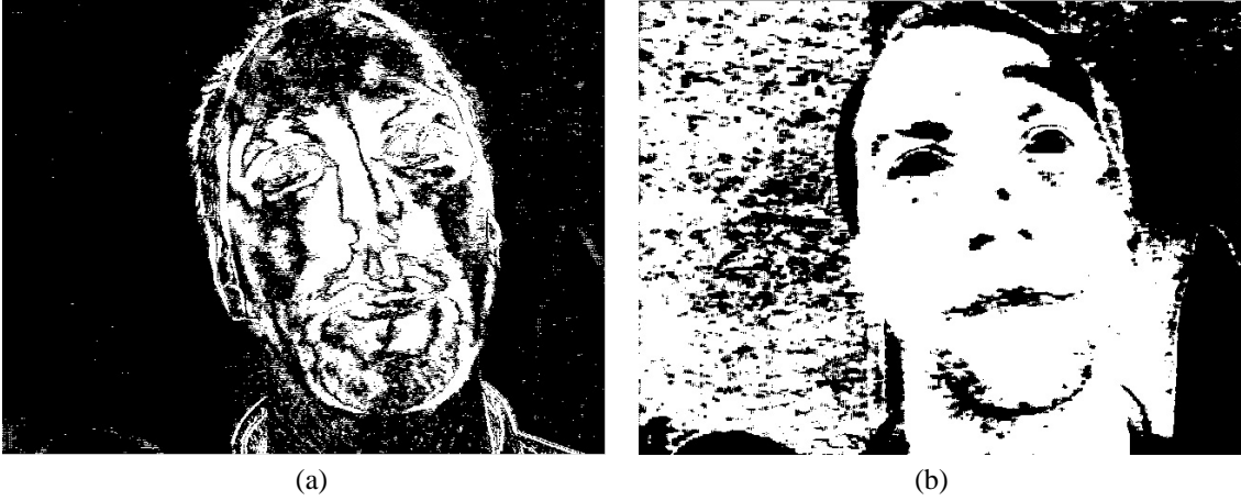
Figure 16: (a) Mask obtained by subtracting images (black pixels are considered as background); (b) Mask obtained by using a face skin color model (white pixels are considered as face skin).
