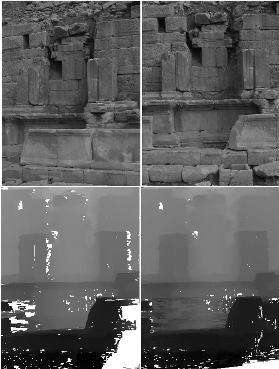
Figure 7.19: First and last image of fountain sequence (left). Depth maps from the 2-view and the 5-view estimator (from left to right) showing the very dense depth maps (right).
