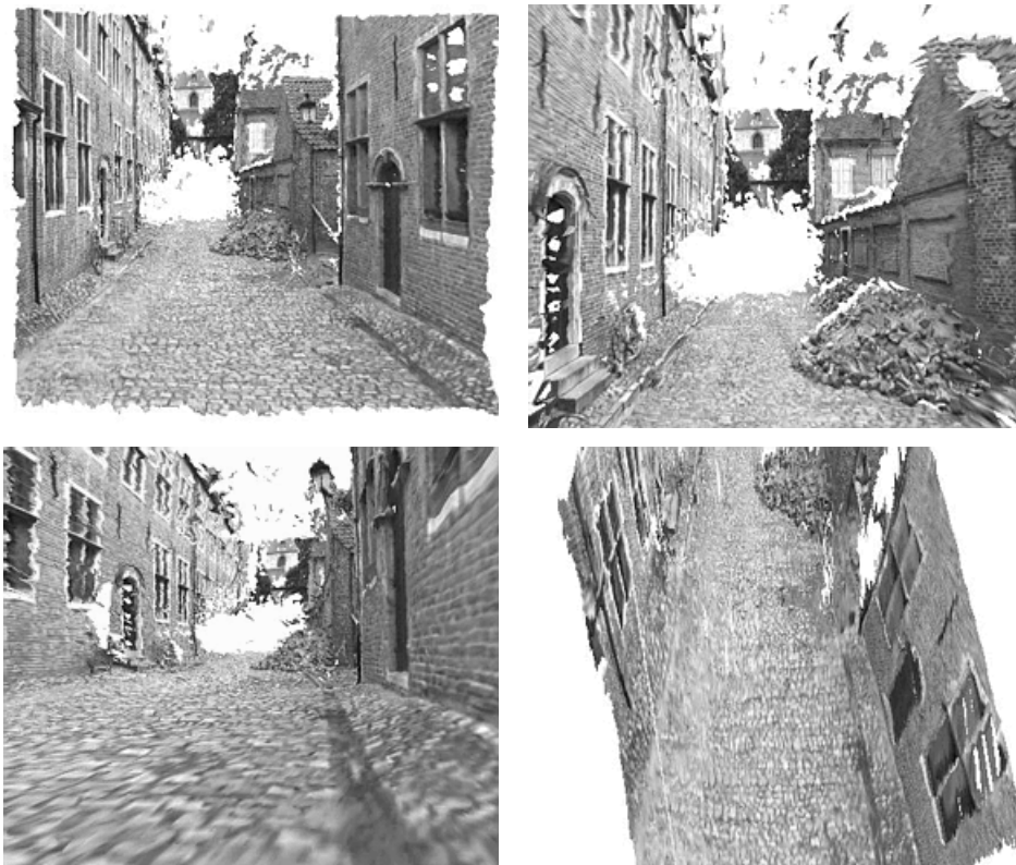
Figure 9.9: Views of a reconstruction obtained by combining results from more images.
