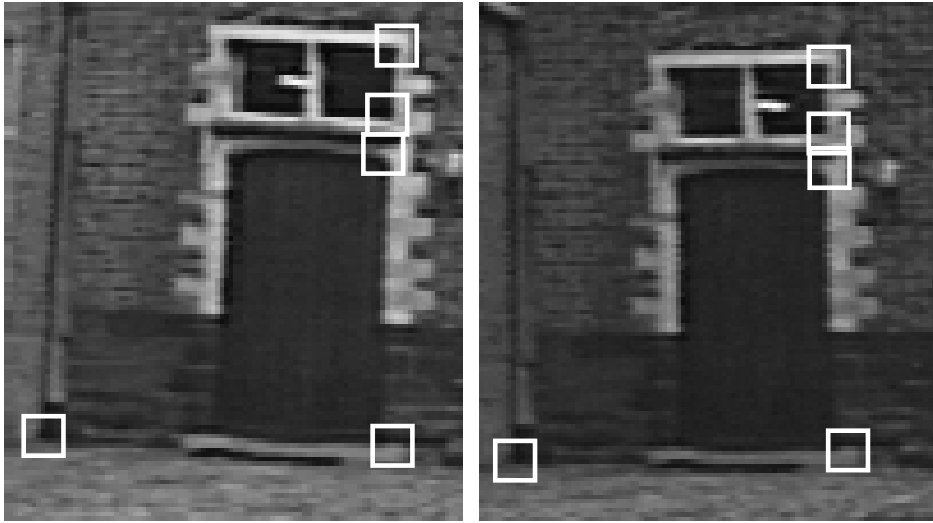
Figure 4.2: Detail of the images of figure 4.1 with 5 corresponding corners.
