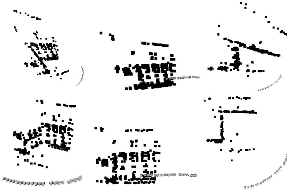
Figure 6.3: Structure and motion before (top) and after (bottom) self-calibration.
