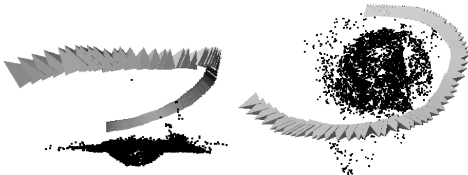
Figure 9.11: The reconstructed interest points and camera poses recovered from the TV sequence.
