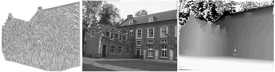
Figure 8.1: Surface reconstruction approach: A triangular mesh (left) is overlaid on top of the image (middle). The vertices are back-projected in space according to the value found in the depth map (right).
