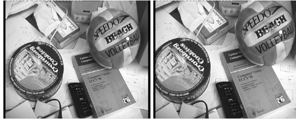
Figure 7.13: Image pair of the author’s desk a few days before a deadline. The epipole is indicated by a white dot (top-right of ‘Y’ in ‘VOLLEYBALL’).
