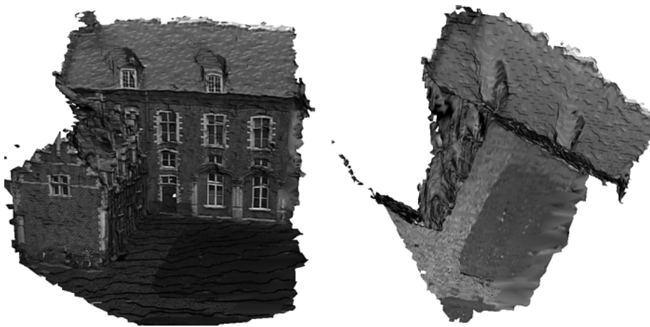
Figure 8.7: Textured surface model obtained through volumetric approach.
