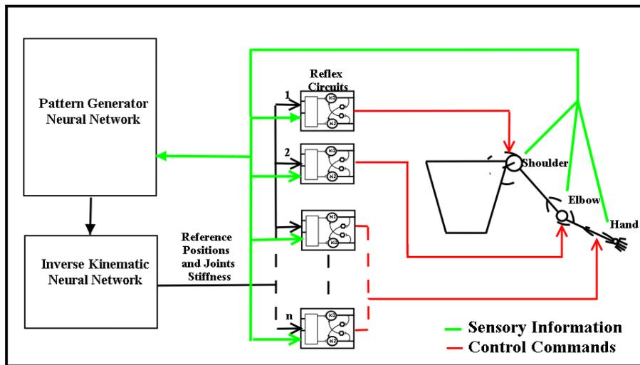
Fig. 2. Control Architecture
