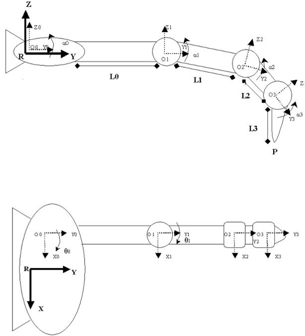
**Fig. 3.** Right hand index, in lateral view
