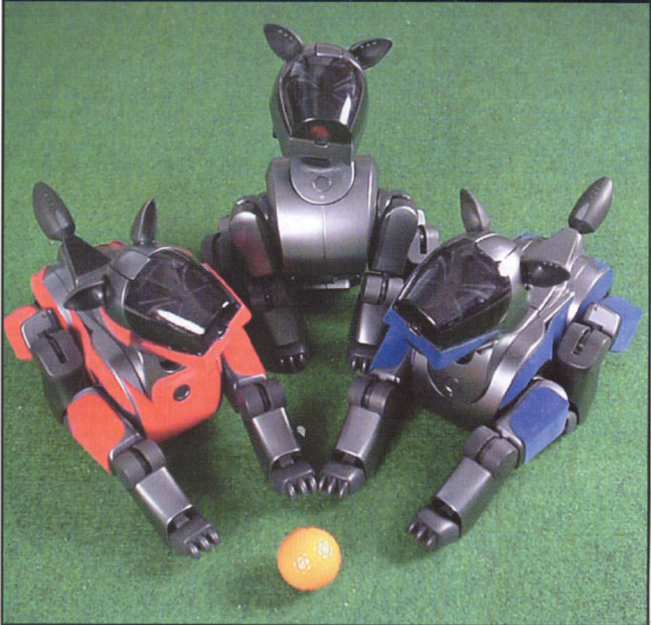
Figure 3. Sony-built Aibos are programmed by Veloso's students to play soccer in teams of three fully autonomous robots.
