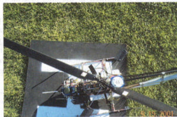
The USC Autonomous Vehicle Aerial Tracking and Reconnaissance (AVITAR) helicopter coming in for an autonomous landing; the craft is not under the radio control of a human pilot.
