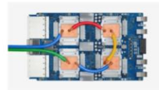
Cloud TPU v3 420 teraflops 128 GB HBM
