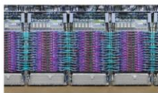
Cloud TPU v3 Pod 100+ petaflops 32 TB HBM 2-D toroidal mesh network
