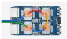
Cloud TPU v3 420 teraflops 128 GB HBM
