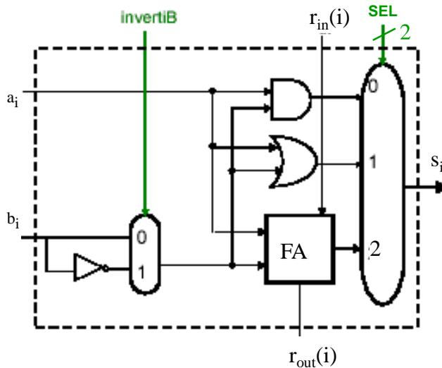
$$r_{in}(i) = r_{out}(i-1) \quad i = 1, 2, 3, \dots, 31$$
