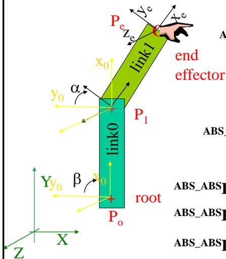
$${}_{ABS\_ABS}P = \begin{bmatrix} l_1 \cos(\alpha + \beta) + l_0 \cos \beta + T_x \\ -l_1 \sin(\alpha + \beta) - l_0 \sin \beta + T_y \\ 0 \\ 1 \end{bmatrix}$$
