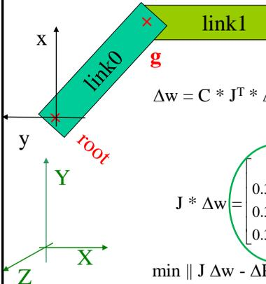
$$\Delta w = C * J^T * \Delta P = \begin{bmatrix} -0.0976 \\ -0.2357 \end{bmatrix} \text{radianti} = \begin{bmatrix} d\alpha \\ d\beta \end{bmatrix} = \begin{bmatrix} -5.593 \\ -13.506 \end{bmatrix} \text{gradi}$$
