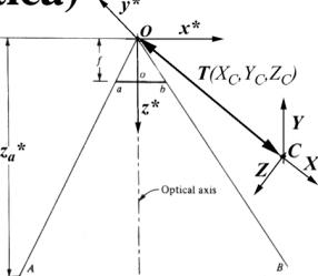
$$(x_a - x_o) / f = X_A^* / Z_A^* = \frac{r_{11}(X_A - X_C) + r_{12}(Y_A - Y_C) + r_{13}(Z_A - Z_C)}{r_{31}(X_A - X_C) + r_{32}(Y_A - Y_C) + r_{33}(Z_A - Z_C)}$$
