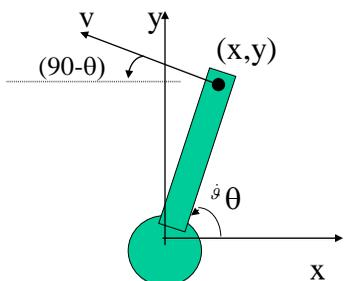
$$\begin{bmatrix} \dot{x} \\ \dot{y} \end{bmatrix} = \begin{bmatrix} \frac{\partial x}{\partial \mathcal{G}} \\ \frac{\partial y}{\partial \mathcal{G}} \end{bmatrix} = \begin{bmatrix} -r \sin \mathcal{G} \\ r \cos \mathcal{G} \end{bmatrix} \dot{\mathcal{G}}_{\mathcal{G}=\theta_k}$$
