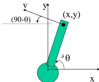
$$\begin{bmatrix} \dot{x} \\ \dot{y} \end{bmatrix} = \begin{bmatrix} \frac{\partial x}{\partial \mathcal{G}} \\ \frac{\partial y}{\partial \mathcal{G}} \end{bmatrix} = \begin{bmatrix} -r \sin \mathcal{G} \\ r \cos \mathcal{G} \end{bmatrix}_{\mathcal{G}=\mathcal{G}_k} \dot{\mathcal{G}}$$
