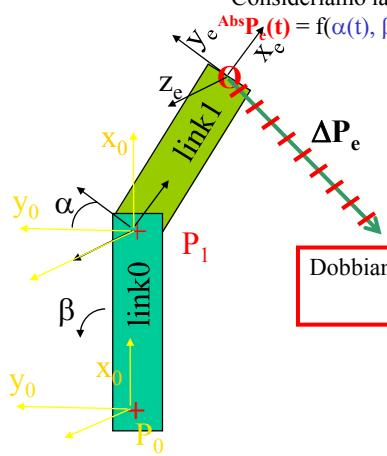
$$\text{ABS\_ABS}P(t) = \begin{bmatrix} l_1 \cos(\alpha(t) + \beta(t)) + l_0 \cos \beta(t) + T_x(t) \\ -l_1 \sin(\alpha(t) + \beta(t)) - l_0 \sin \beta(t) + T_y(t) \\ 0 \\ 1 \end{bmatrix}$$
