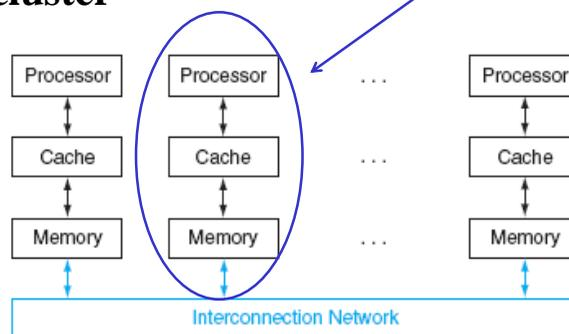
Synchronization through **message passing** multiprocessors (sender – receiver).
