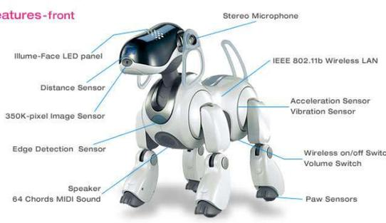
Labels for AIBO robot features: Stereo Microphone, IEEE 802.11b Wireless LAN, Acceleration Sensor, Vibration Sensor, Wireless on/off Switch, Volume Switch, Paw Sensors, Speaker, 64 Chords MIDI Sound, Edge Detection Sensor, 350K-pixel Image Sensor, Distance Sensor, Illume-Face LED panel.
