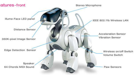
Labels for AIBO robot features: Stereo Microphone, IEEE 802.11b Wireless LAN, Acceleration Sensor, Vibration Sensor, Wireless on/off Switch, Volume Switch, Paw Sensors, Speaker, 64 Chords MIDI Sound, Edge Detection Sensor, 350K-pixel Image Sensor, Distance Sensor, Illume-Face LED panel.
