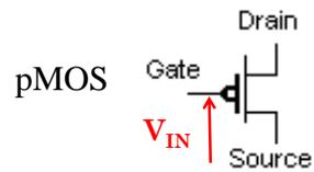
Accesso se:  $V_{in} < V_{dd}/2$
