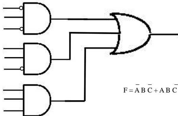
$$F = \bar{A}\bar{B}\bar{C} + A\bar{B}\bar{C} + A\bar{B}C$$
