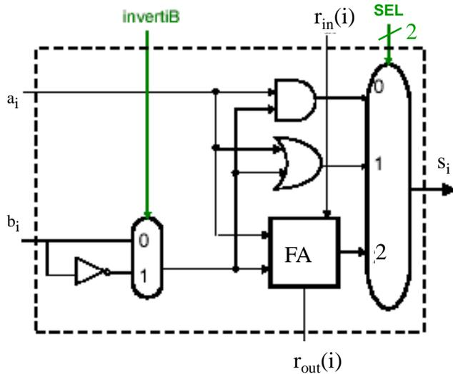
$r_{in}(i) = r_{out}(i-1)$   $i = 1, 2, 3, \dots, 31$
