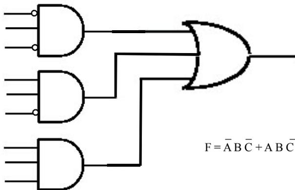
$$F = \bar{A}B\bar{C} + A\bar{B}\bar{C} + ABC$$
